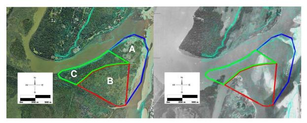
Figure 4.5. Approach recommended for the phased removal of dredge spoil that had been historically dumped between the uMfolozi mouth and the St Lucia Narrows. The "Combined mouth" scenario evaluated in the GEF study (Clark et al. 2014) corresponded with the removal of dredge spoil in area A (diagram on left) while in the "Reference" state it was assumed that sediment had been removed from all three compartments as per the 1937 configuration on the right.
