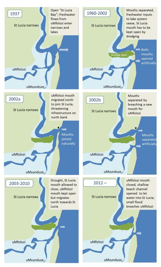
Figure 4.1. Changes in the structure and functioning of the mouth of the Lake St Lucia estuary system (Source: Clark et al. 2014b).
