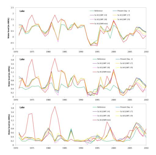
Figure 6.9. Variation in water level in the Lakes (top), Narrows (middle) and the uMfolozi (bottom) with the Beach channel under reference and presentday conditions and under the operational flow scenarios.
