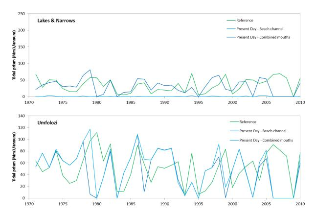
Figure 4.9. Tidal flows up the Narrows and uMfolozi channels for the Reference and Present Day. Note that Present Day conditions have been modelled as two separate scenarios – Mouth A with the existing beach channel in place and Mouth B after Phase 1 of the dredge spoil removal process has been completed.
