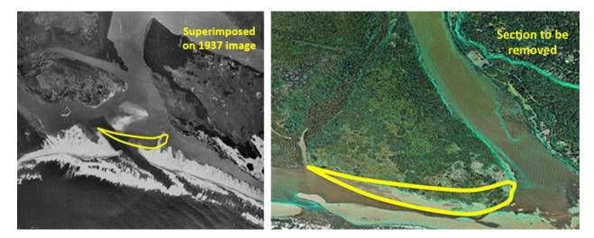
Figure 4.4. The mouth of the Lake St Lucia system in 1937 (left) and as it is at present (2013, right). The 2013 photograph shows the dredge spoil material that was placed in the river course from the 1950s for a period to try and separate the uMfolozi River from Lake St Lucia. The yellow boundary shows the first portion of dredge spoil that will be removed as part of Phase 1 of the restoration action.
