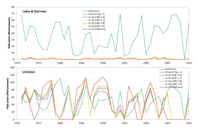
Figure 6.7. Variation in tidal inflow volume up the Narrows (top) and the uMfolozi channel (bottom) with the Beach channel (Mouth A) under reference and present-day conditions and under the operational flow scenarios.
