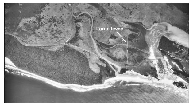
Figure 4.15. Aerial photo from June 1960 showing the larger levee (constructed in 1957-1960) and further straightening of the uMfolozi channel. (Source: Illenberger & Clark 2014).
