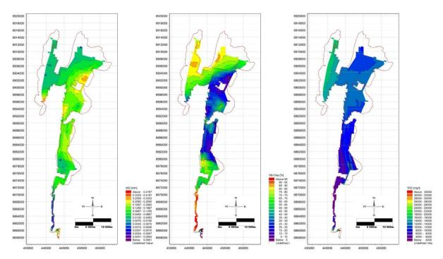
Figure 4.10. Spatial distribution of the median diameter of bed sediments (left) and percentage clay, silt (middle) and near surface TSS concentrations (right) as measured during March 2013 (Source: Basson *et al.* (2014).
