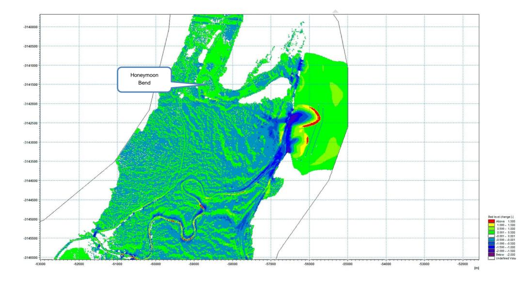
Figure 4.19. Model simulations showing change in bed level around Honeymoon Bend following a 1:100 year flood (Source: Basson *et al.* 2014).
