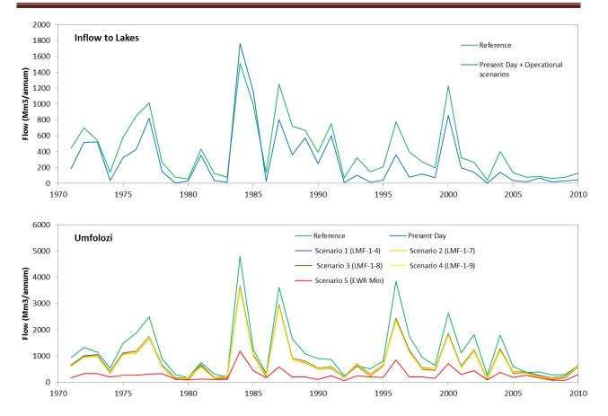
Figure 6.4. Inflows directly to the Lakes (top) and down the uMfolozi (bottom) under reference and present-day conditions and under the operational flow scenarios. Note that inflows directly to the St Lucia Lakes are the same for all operational scenarios.
