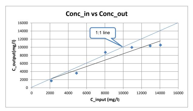
Figure 4.12. Simulated sediment transport from upstream to downstream of the uMfolozi floodplain by the 2D hydrodynamic model for different flood hydrographs (Source: Basson *et al.* 2014).
